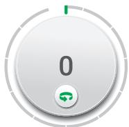
1. Tap the reverse symbol on the speed dial to switch the rotating direction of the mixing knife from forward (clockwise) to reverse (counter-clockwise).
