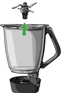
1. Ensure that the sealing ring of the mixing knife is correctly positioned under the knife bearing.
